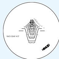
No.12AAG849 (MF D)*2 Involute gear reference rack m = 0.1 to 1.0, pressure angle: 14.5° Line width: 7μm
