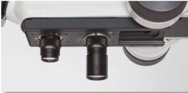
Sliding nosepiece with two objectives mounted.
